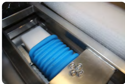
Water-resistant, encapsulated silicone-coated loadcell
