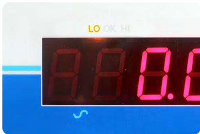
'Hidden until lit' checkweighing lights show if weight is above, below or within limits
